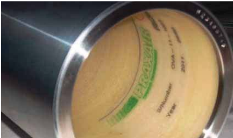
The new generation of sleeves have stainless steel rings on both ends and sealing of the composite face in order to improve resistance to cleaning and increase lifetime
