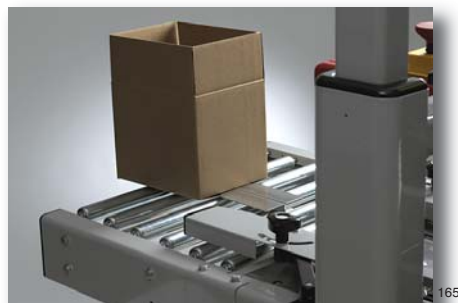
Box Hold Down Attachment – Holds RSCs on the optional infeed conveyor to free the operator's hands for cases filling.
