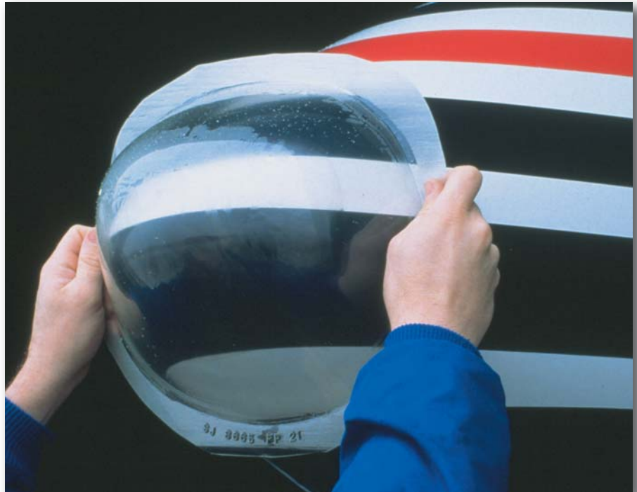
Aircraft radomes are protected against particle and rain erosion with transparent 3M™ Preformed Boots. The boots conform and adhere on contact to the curvature.
