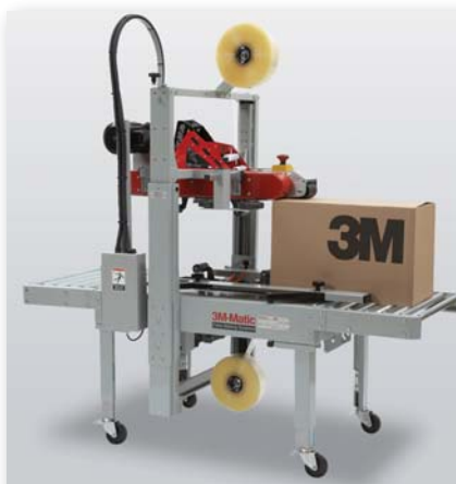
700a – Advanced features to seal uniform cases up to 40/minute. Dual masts with dual lead screws for stability and uniform height adjustments. Adjustable top and bottom belt drive system for reliable conveyance of heavier or tall/light boxes. Compression rollers position each box for precise tape sealing.
