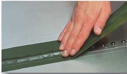
3M™ Vinyl Tape 471 conforms to seal riveted seams. The flexible backing shapes itself to the bumps and edges, and the rubber adhesive holds securely to the metal.
