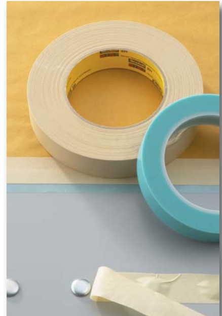
3M™ Fine Line Masking Tape 4737T applied over the edge of 3M™ Crepe Masking Tape 231, provides a sharp line for painting a truck panel. The crepe tape holds gross masking product in place.
