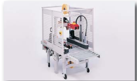
800r – Automatically adjusts for case size. Self-centering side belt drive for consistent flow of narrow cases at up to 19/per minute. 36 mm to 48 mm wide tapes.
