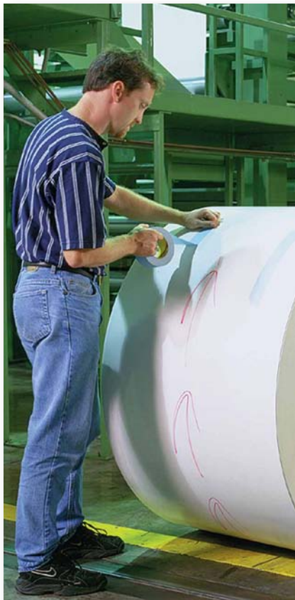
High tack 3M™ Temporary Single Coated Repulpable Tapes are available in white, blue, and kraft for dependable core starting, roll closing, and butt splicing.
