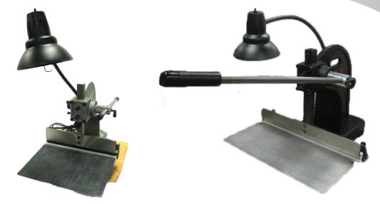
The features of these plate cutters alleviate lost time searching for razor blades to accurately cut your flexo plates. The flexible work lamp provides intense lighting where needed to ensure accurate cuts, and the work table grid allows for easy alignment with see-thru photo-polymer plates registration marks. Beveled cuts are made simple by the design of the blade for butt joints on reverse printing plates, so you dont even have to tilt the table!
